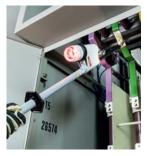
The compact design of the PHE4 voltage detector is beneficial in **electrical switchgear assemblies**.
