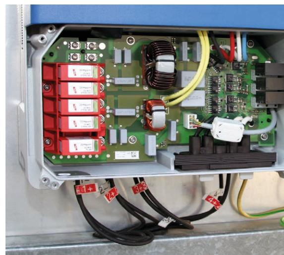
Figure 9 DEHGuard type 2 SPD integrated in the inverter for the DC side
